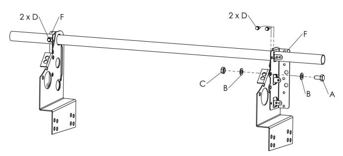
The ridge rail is designed and rated for the attachment of one person with personal fall protection equipment.
